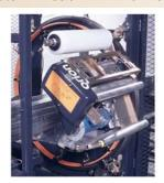
The Constellation is equipped with the Insta-Thread™ powered pre-stretch film delivery system and is compatible with all high quality stretch films from 10″ to 30″ in width.
