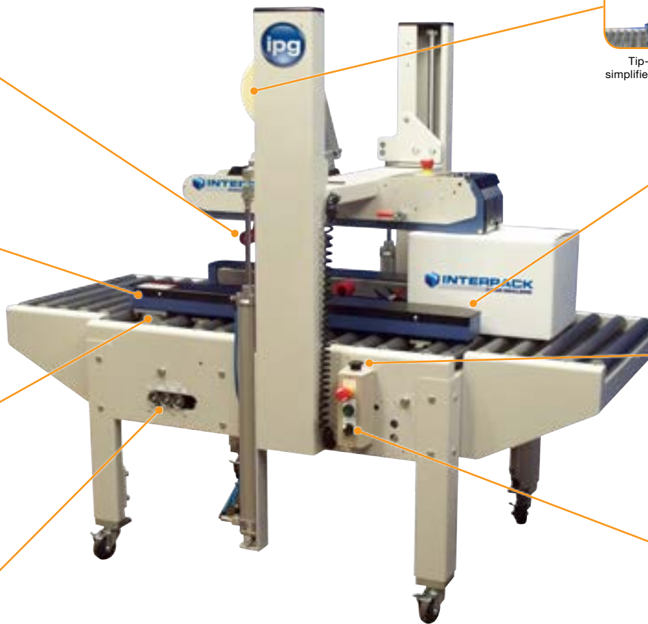
Offset tape heads process 2" high cases
