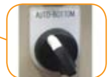
Top & bottom or bottom only seal operation modes
