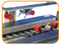
Offset tape heads process 2" high cases
