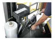
All Flex LPA's are equipped with the Insta-Thread<sup>™</sup> film delivery system and film tail treatment mechanism with drop-in film loading for fast, easy and safe threading of film.
