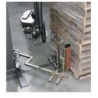
At the end of the wrapping cycle, an innovative asymmetrical film clamp grips the film while the impulse wire cuts the film. The load seeking brush then presses the film tail to the side of the load.
