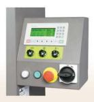
The Sentry control panel features a multi-language display, knobs for turntable speed, carriage speed, and film tension, power light, start button, E-stop button and power disconnect.
